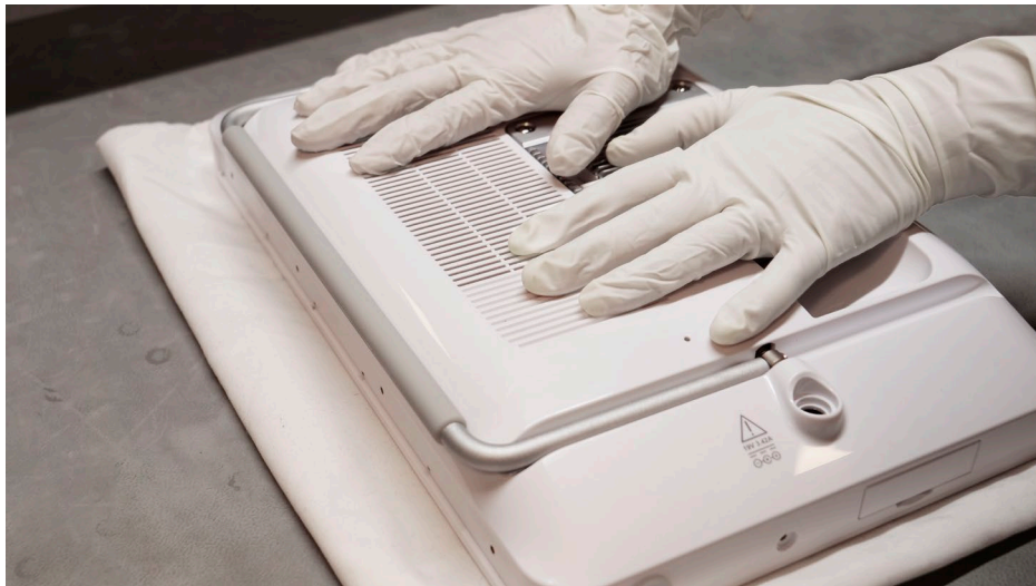
Figure 32 Put on the back casing till it clicks in place
