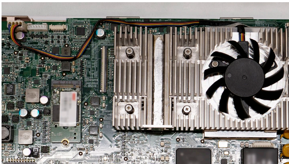
Figure 25 Install the fan
