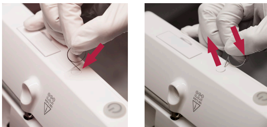
Figure 5 Removing the screw cover
